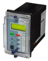
ARGUS overcurrent relay Directional, size 4 molded case, 4 CT, 3 VT, 10 LEDs, 9 binary inputs/ 6 binary outp. Measuring input: 1/5 A, 50/60 Hz with SEF input, 63.5/110 V auxiliary voltage: 60 to 240 V AC/DC, binary input threshold 88 V AC/DC Standard version - no cover Communication: front port: USB and rear: RS485 supporting IEC 60870-5-103 or MODBUS RTU or DNP 3.0. . Front fascia: w. breaker control pushbuttons protection function: standard version
