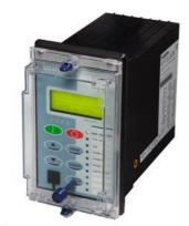
ARGUS overcurrent relay Non-directional, size 4 molded case, 4 CT, 10 LEDs, 6 binary inputs/ 6 binary outp. Measuring input: 1/5 A, 50/60 Hz with SEF input auxiliary voltage: 24 to 60 V DC, binary input threshold 19 V DC Standard version - no cover Communication: Front port: USB and rear: RS485 supporting IEC 60870-5-103 or Modbus RTU or DNP 3.0. . Front fascia: w. breaker control pushbuttons protection function: standard version
